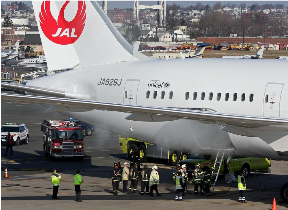
Figure 1. Smoke emanating from the aft electronic equipment bay. Source: Boston Herald .
