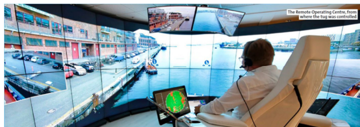
Remote Control Svitzer Hermod Bridge— Rolls-Royce / Svitzer Remote Operating Center, Copenhagen
