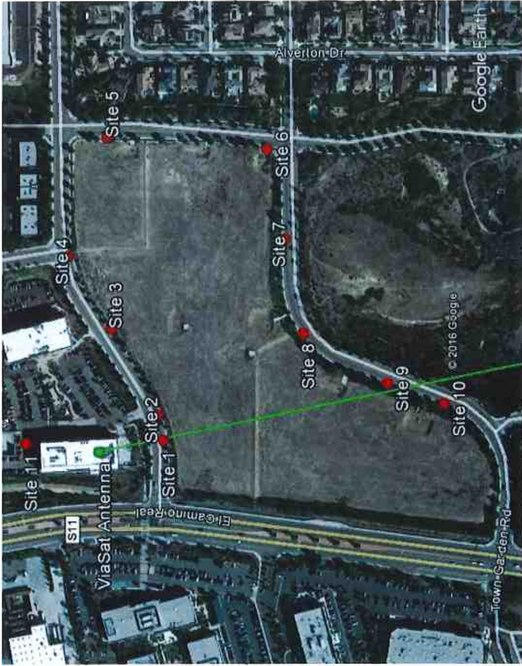
The green line is the main beam azimuth. Red dots show measurement locations,
