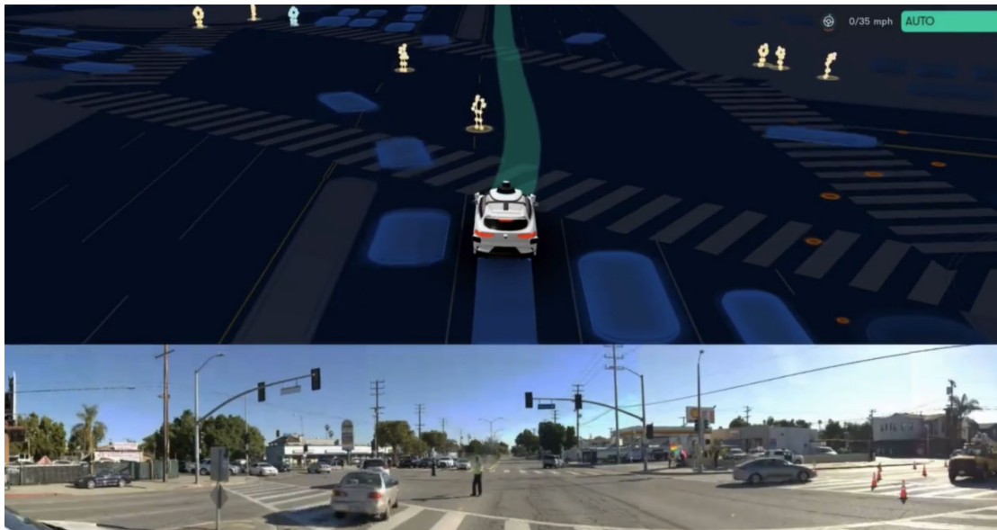
A Waymo vehicle recognizes and adheres to a police officer directing traffic at a Los Angeles intersection. 30
