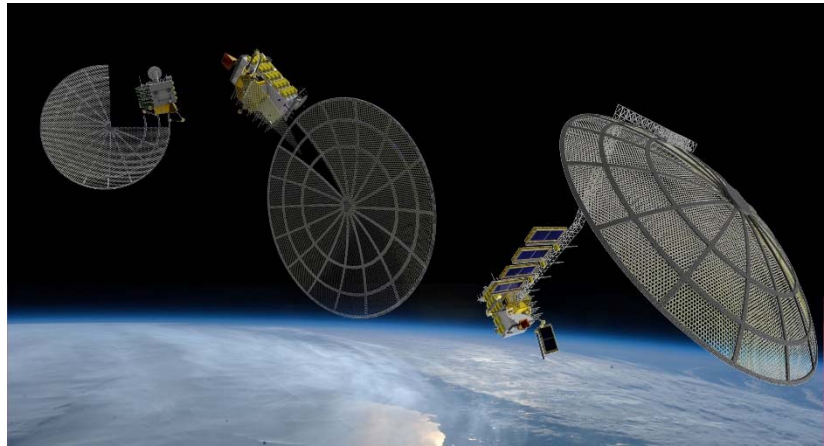
Figure 3. This artist's rendering depicts the Archinaut payload during its deployment in space. Via additive manufacturing and assembly, a large reflector is manufactured and integrated over time. Image credit: Made In Space
