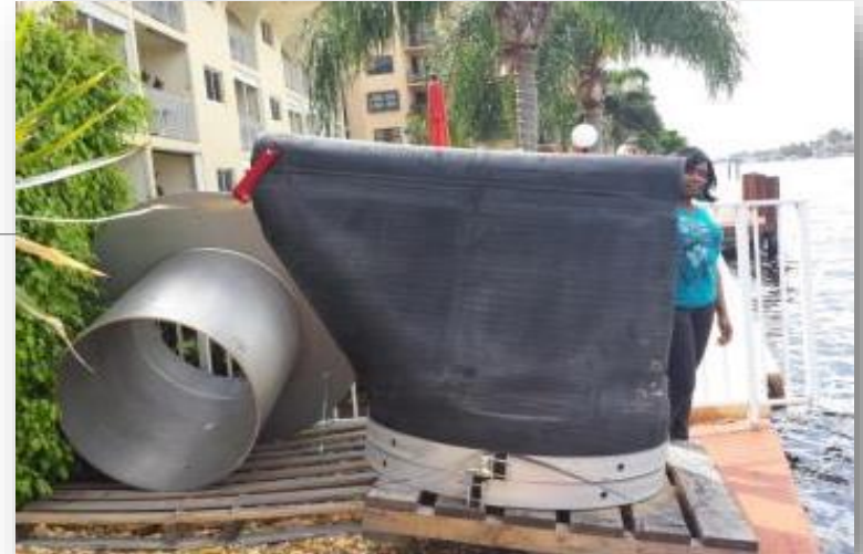
Stormwater valve – Pompano Beach, FL
